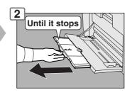
Adjust the width guides. Incorrect adjustment may cause the paper to wrinkle, misfed, or skew.
